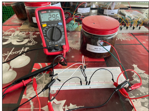
Figure 2. Measuring voltage and current generated by the SMFC using a multimeter
